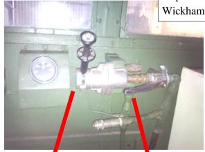
Above Air Dump Valve (normal running) Pull Collar and lower valve to dump air.
